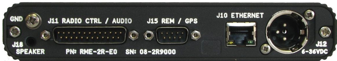
Fig2: Rear panel of the RM2-HVM Unit
