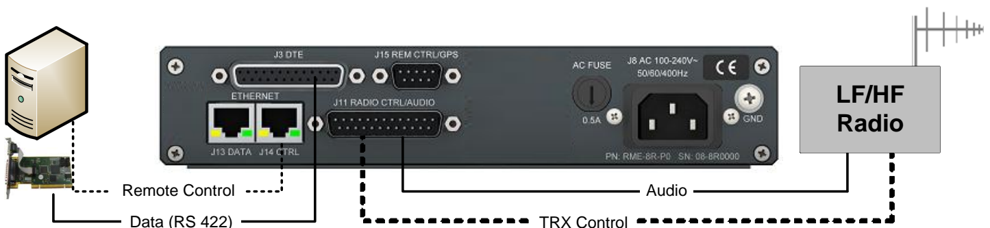
Figure 1: Rear Panel connections on RM6-A –Variant 1: AC PSU RapidM (RM-SC sync card also shown)
