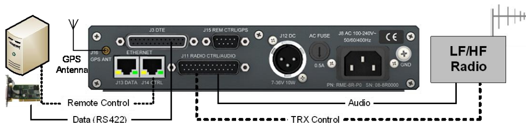
Figure 1: Rear Panel connections on RM8 – Variant 2: AC + DC PSU ( RapidM RM-SC sync card also shown)
