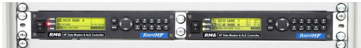
Figure 2: Two RM6 Units side-by-side in a 19-inch rack
